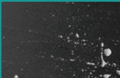
↑ Overview of cavitation damage zone after 720 min. exposure time. More and bigger delaminations. Undulations in the coated areas are clearly visible.
