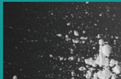
↑ Overview of cavitation damage zone after 1080 min. exposure time. Failed areas coalesce.
