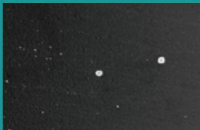
↑ Overview of cavitation damage zone after 270 min. exposure time. Failed area is very small.
