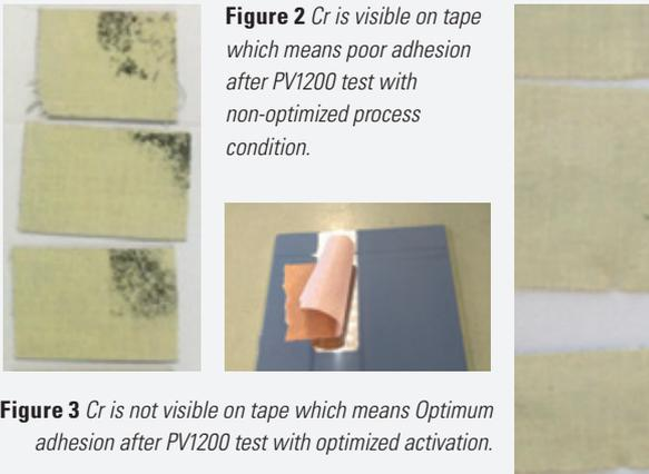
**Figure 2** Cr is visible on tape which means poor adhesion after PV1200 test with non-optimized process condition.
