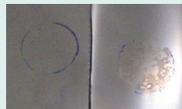
**Figure 6** Performance of Cromatipic® (left) and electroplating (right) in Russian Mud Test
