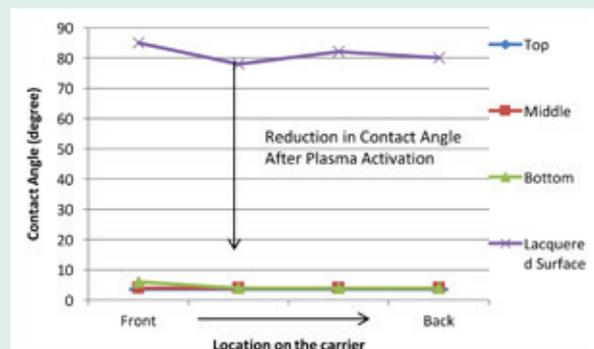
**Figure 1** Uniform water contact angle with different height and width for a carrier front to back
