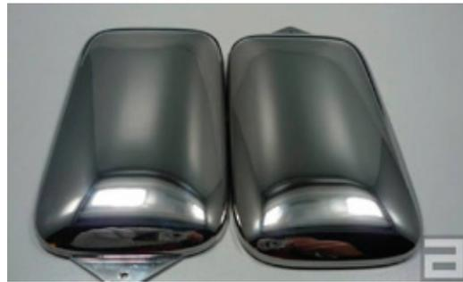
**Figure 5** Optimum corrosion resistance on Cromatipic® sample after CASS test
