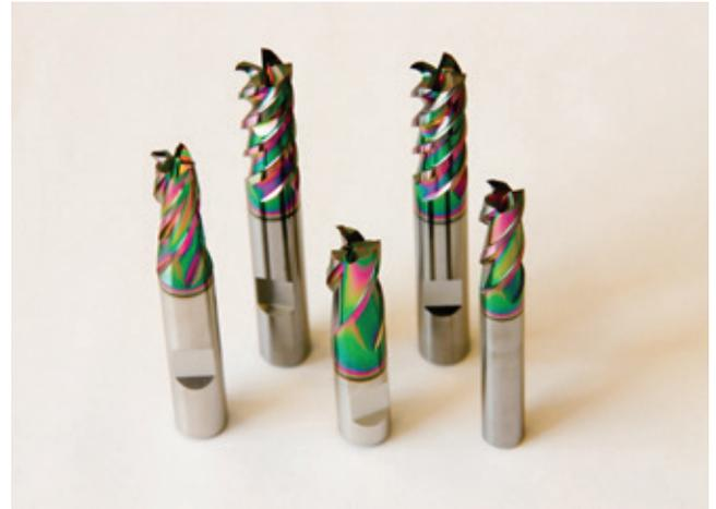
coatings. With the introduction of the latest generation of power supplies and the possibility to program pulse trains with pulse width modulation, Hauzer's HiPIMS technology is now also suitable for target materials such as graphite, making the deposition of hard hydrogen-free carbon coatings with HiPIMS a reality.
